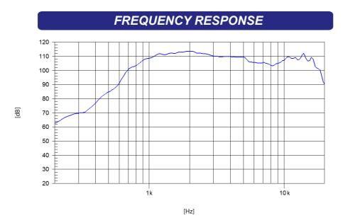
Note: On axis frequency response measured coupled to TD-365 horn in anechoic chamber, 1W / 1m
